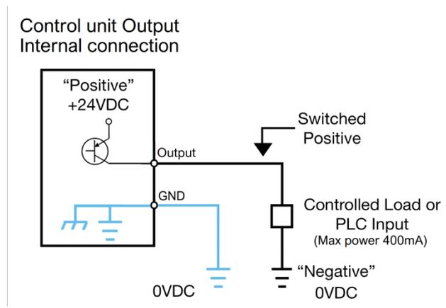
These pins can be used directly connected to PNP inputs (PLC) or used to turn on LEDs, buzzers or other devices with 24V power supply. The maximum total power of the outputs is about 400mA. Using inductive loads such as relays or other loads with an initial consumption peak greater than 400mA will send all outputs to protection, displaying the message "output disable". To restore the outputs after a protection, turn off and turn on the unit again.
