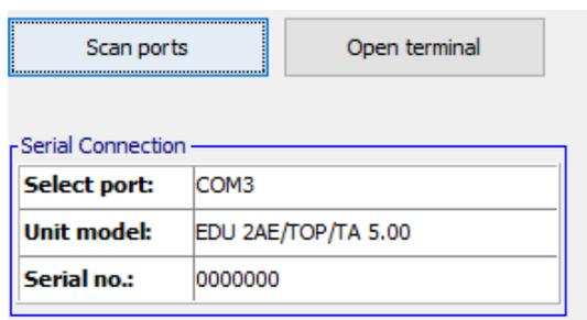
Click *Scan ports* to locate the unit. EDU EXPAND recalls the port, the model of the control unit and its serial number. Then click *Upload to unit*. The text *Programming...* will appear on the EDU display. When the text *Programming...* disappears, you may disconnect the cable. Uploading can only be initiated if the control unit shows *Ready* on the main screen.
