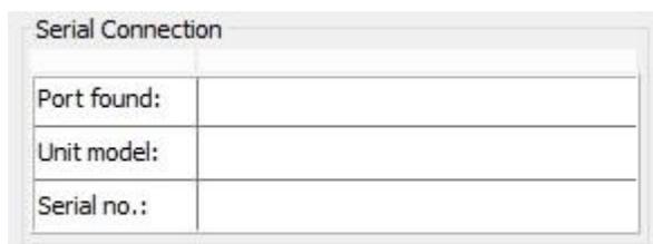
The control unit must be connected to the PC via miniUSB port or RS232 seat in the back panel of the unit.
