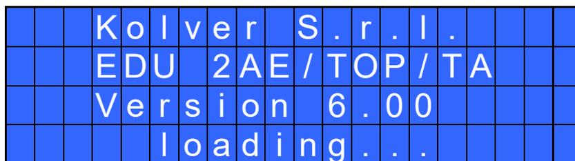
When turned on and the screwdriver is connected, the unit is set to % mode and the display will contain the following information:
